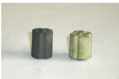
Figure 9: Ni / CaAl 4 O 7 catalyst in the uncracked part (left) and cracked part (right)
