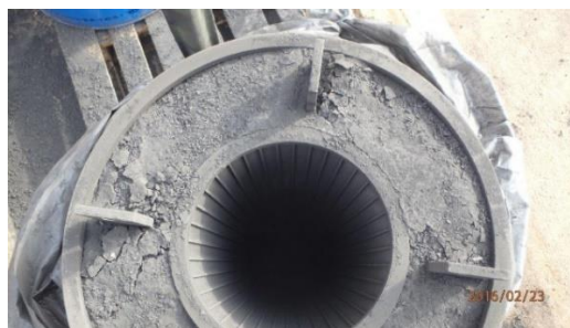
Fig. 10. Black deposit inside the internal reactor tubing.
