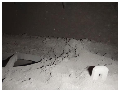
Fig. 11. Black deposit on catalytic bed of the reactor.
