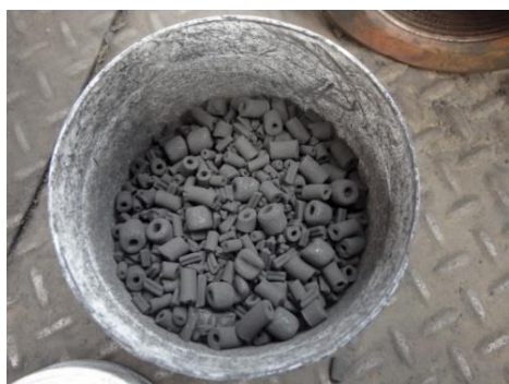
Fig. 9. Black deposit on the inert catalyst.
