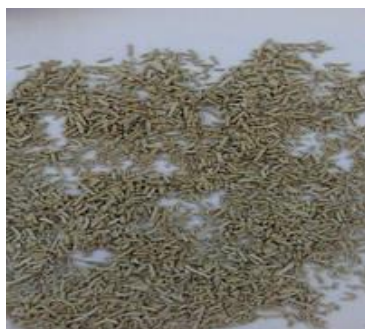
Fig. 8. Oxyded form of the catalyst NiMo/Al 2 O 3 .
