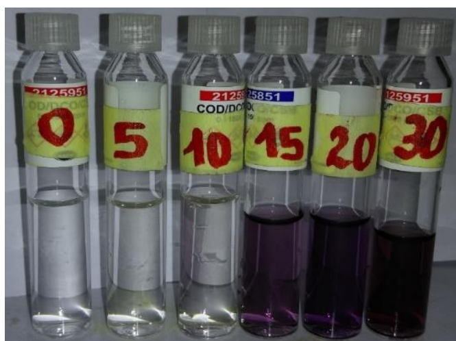
Fig. 8. Starch test for the demonstration of diiodine formation during electrolysis of the TLX solution.
