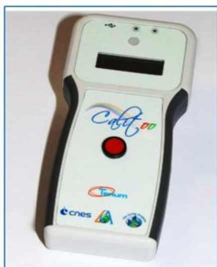
Fig. 2. Calitoo Sun Photometer.
