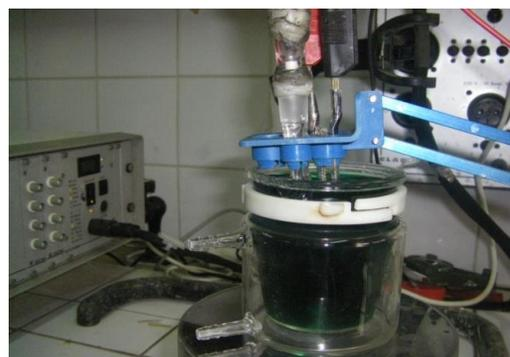
**Fig. 2.** Electro deposition apparatus.
