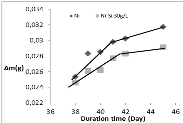
**Fig. 8:** Zoom on the catch of mass of the patterns coated with nickel and the Ni/Si 30g/L electrolytes from the thirty eights day.
