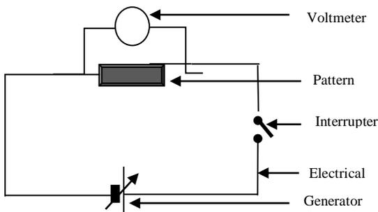
**Fig.5.** Resistance measurement apparatus.
