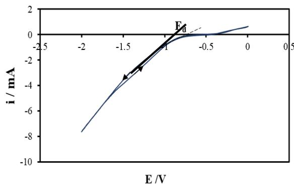
**Fig. 3.** The cyclic voltammety registration for nickel reduction obtained on carbonaceous steel.
