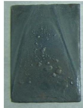
**Fig.7.** Witness pattern aspect after thermal treatment.
