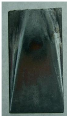
**Fig. 12.** The Ni coated pattern after the thermal treatment and exposure to atmosphere.
