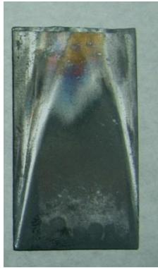
**Fig. 11.** The Ni-Si 50 g/L pattern coated after the thermal treatment and exposure to atmosphere.
