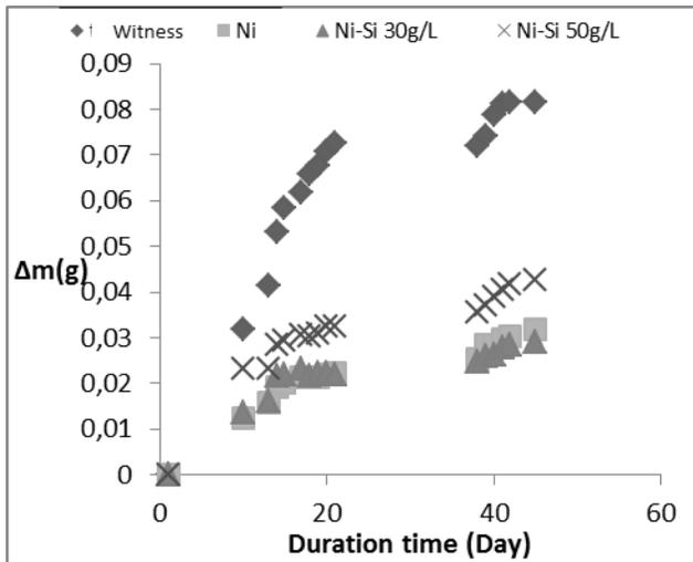
**Fig.6.** Catch of mass of the patterns after thermal treatment and exposure to atmosphere.
