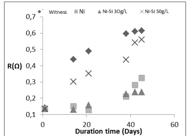
**Fig. 9.** Resistance variation versus the treatment duration.
