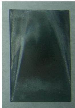
**Fig. 13.** The Ni-Si 30 g/L coated pattern after forty five days of thermal treatment and exposure to atmosphere.
