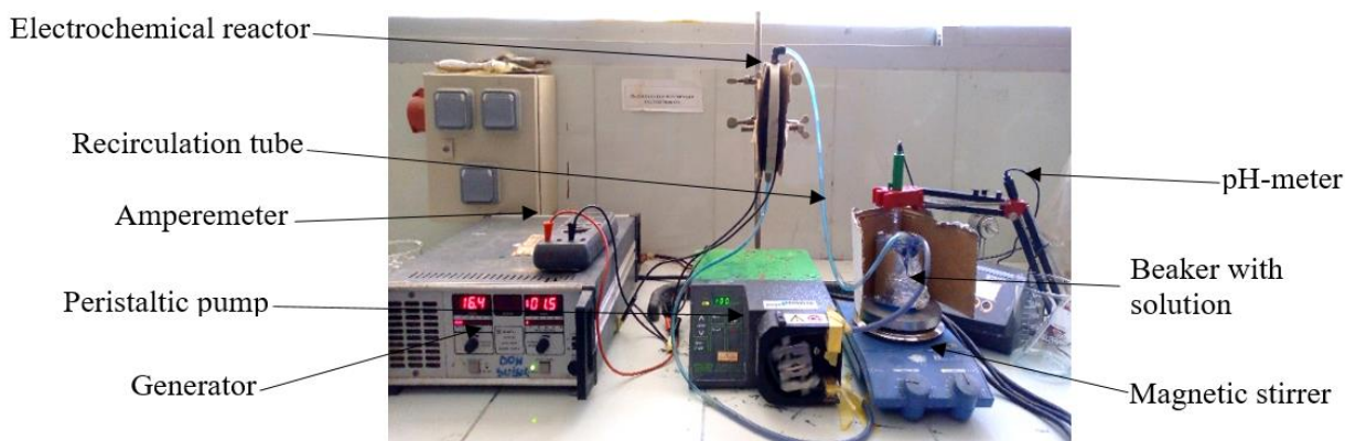
Fig. 1: Device for preparative electrolysis.
