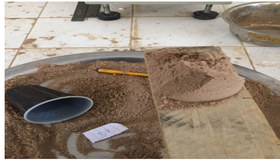
Figure 2: Sand with grains free from capillary forces.
