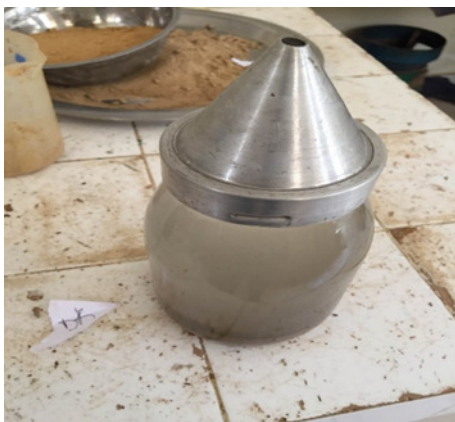
Figure 5: Mass of the pycnometer, water and crushed sand.
