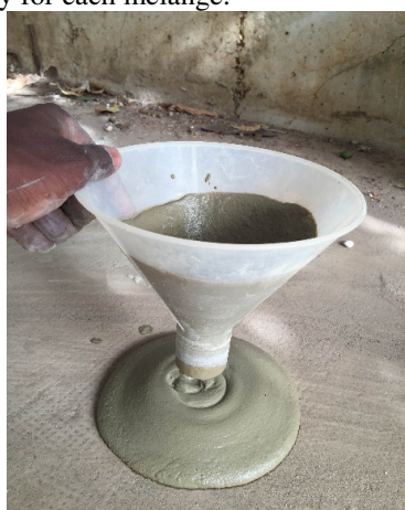
Figure 8: Measure of the workability of the sand concrete (sand of Thiès).
